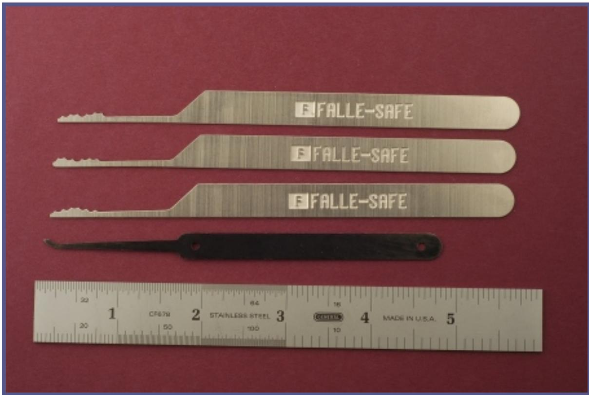
Figure 8. Falle-Safe "rake" picks.
