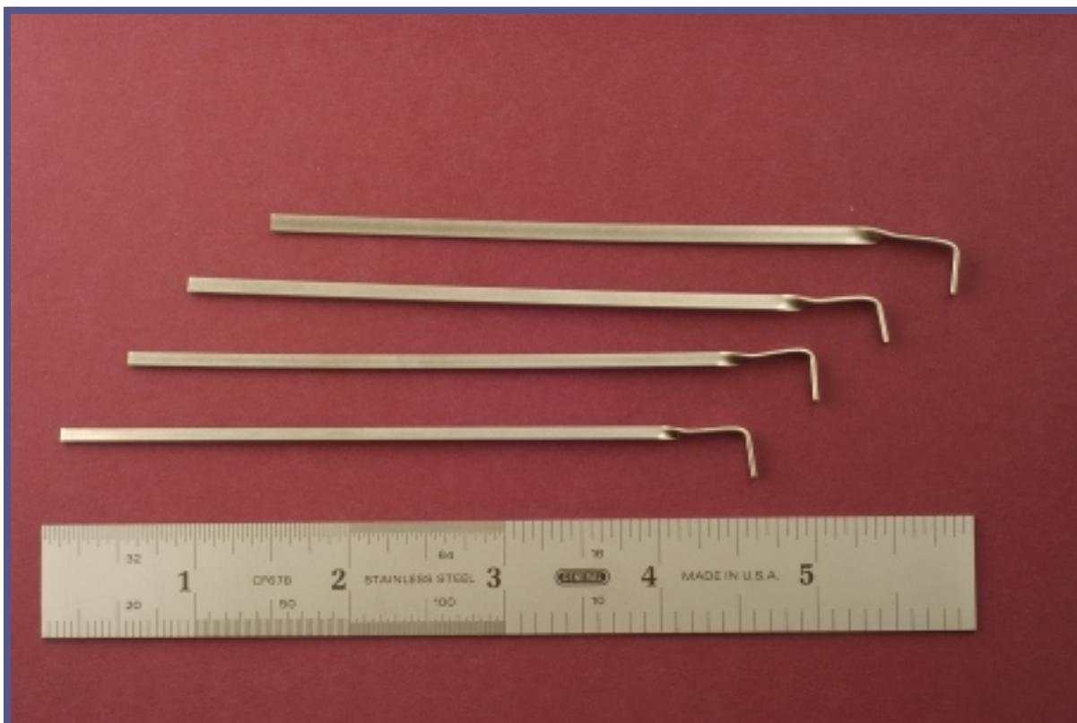
Figure 15. Falle-Safe conventional torque tools (twisted).
