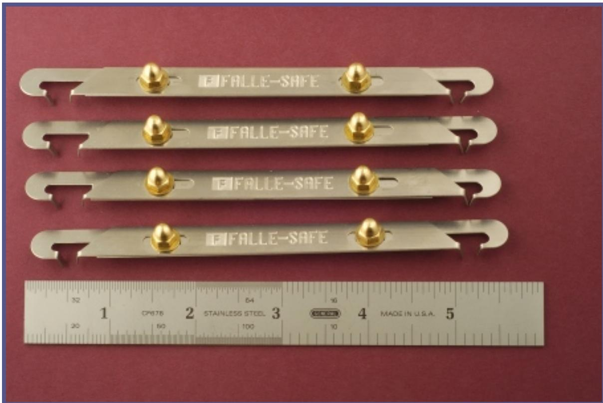
Figure 20. Falle-Safe variable torque tools.
